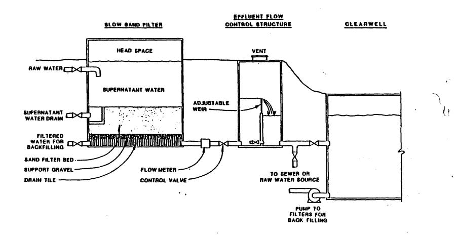
Figure 1. TYPICAL COVERED SLOW SAND-FILTER INSTALLATION
