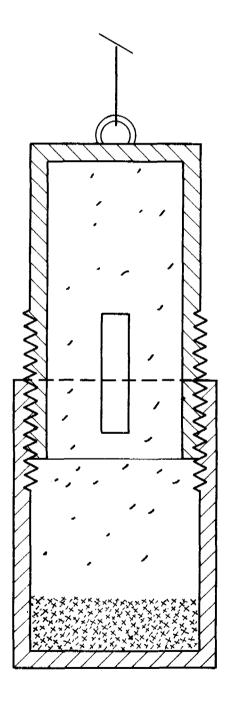
control the iodine feeding at a fixed constant rate. The dissolving iodine forms a solution of high specific density and is concentrated at the bottom of the feeding tube (see figure 4.1.). The dosing rate decreases after a short time and soon becomes too low for practical application.
