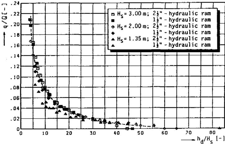
Fig. 8 Flow ratio versus head ratio
