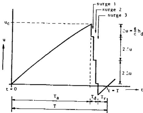
Fig. 3 Velocity  $u(t)$  at the downstream end of the drive pipe
