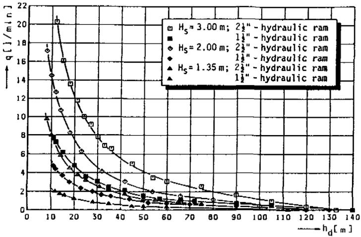
Fig. 7 Effect of ram size on ram performance,
