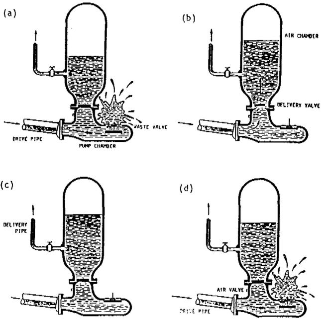
Fig. 2 Operation of the hydraulic ram
