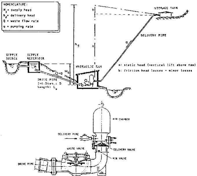
Fig. 1 Typical hydraulic ram installation
