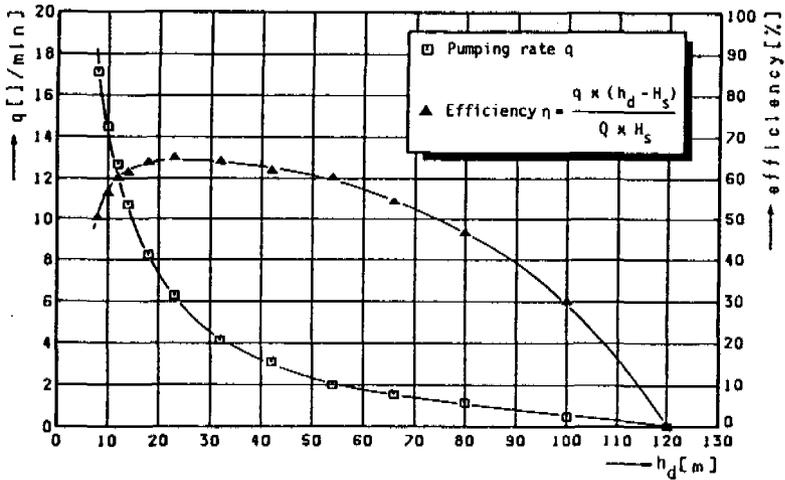
Fig. 5 Performance characteristics, 2 1/2"-hydraulic ram
