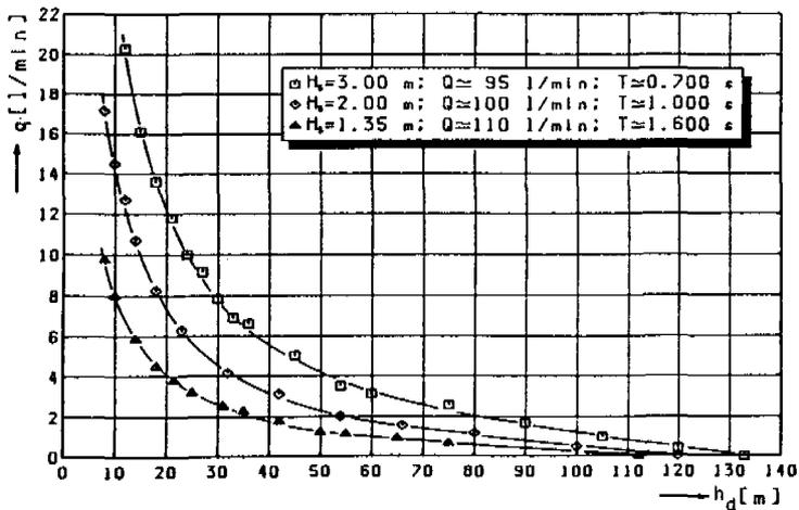
Fig. 6 Effect of supply head on ram performance, 2 1/2"-hydraulic ram
