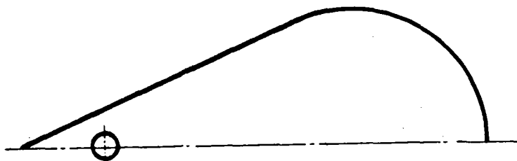
FIG. 7. The shape of Bach's non-cylindrical blade.
