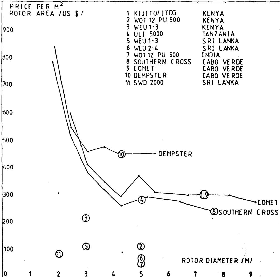
The price of a windmill per square metre of rotor area is a measure of the cost effectiveness. In table 1 the price per square metre of rotor area is given for a number of water pumping windmills. Prices are given for windmill + pump, excluding installation costs.
