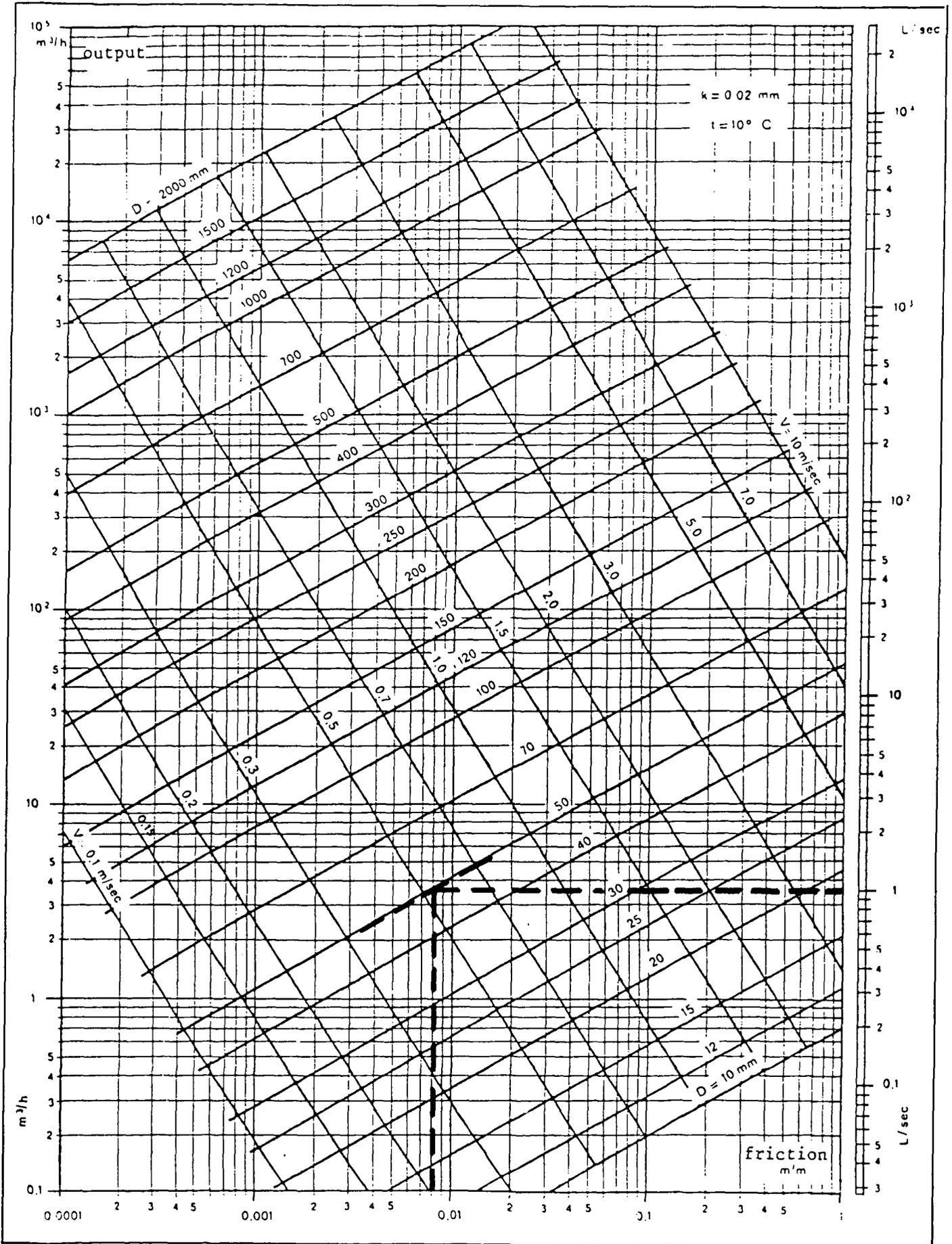
**Example:** the flow of 1  $l/s$  through a PVC or PE pipe with a diameter of 50 mm results in a head loss (friction) of 0.008  $m/m$ . The head loss over 100 m is therefore 0.8 m.
