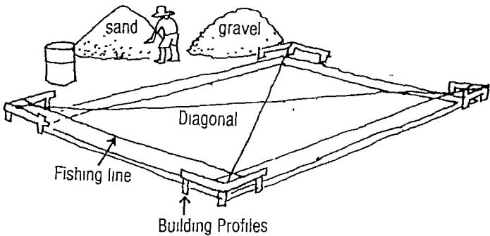
27. Using a line-level attached to the string line will indicate whether the profiles are set to the same height.
