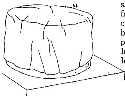
63. The tank should be covered with wet sacking or polythene sheeting to prevent it from drying out too quickly which would cause cracking in the walls. The walls should be kept damp by moistening under the polythene or by keeping the sacks damp for at least two weeks. Materials such as banana leaves can also be used.
