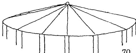
70. To complete the tank, the roof formwork is prepared and assembled, on which reinforcing mesh and wire are laid and plastered with 50 mm of mortar.
