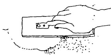
91. Plaster on a second layer to both the inside and outside of the tank. Using a steel float, trowel this to a smooth finish. After 24 hours the floor of the tank can be finished off. Mortar is passed through the manhole, spread over reinforcement to the required thickness and trowelled to a smooth finish.
