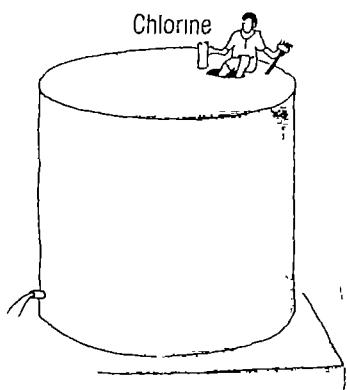
74. The manhole should be screened to prevent insects or dirt from gaining access to the tank. The opening is also used as the discharge point for the rainwater.
