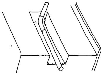
32. From a suitable point within the planned circular wall of the tank, prepare a shallow trench to the outside of the base to a point where outlet will discharge. Lay a length (about 300 mm) of 20 mm pipe with bend and upstand within the trench. (If a drain is provided this should be placed at the same time) See also clause 67
