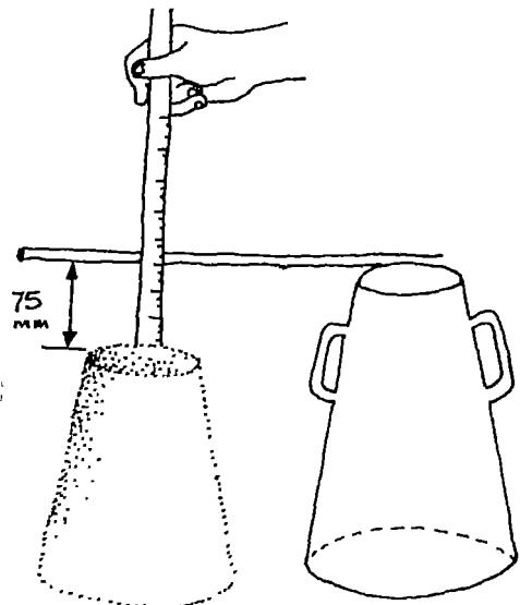
56. The measured slump should be between 75 to 85 mm. If less, add more water to the mix. If more, use less water. With practice it should not be necessary to test every mix particularly if consistent volumes of materials are used.
