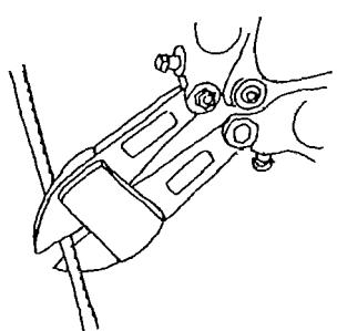
82. A simple jig can be made by fitting 3 short pieces of 25 mm rod into a thick board. Accurate bends and offsets can be reproduced on the bending table. Cutting of rods is best done by using compound action bolt cutters. Alternatively a hacksaw can be used.
