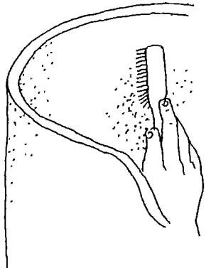
66. To effectively seal the tank, a 2-4 mm coat of *cement slurry* (cement and water), should be brushed or wiped over the internal and external surface of the tank.
