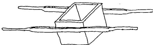
37 To produce a consistent and uniform mix all materials should be measured by volume. This can best be done by using a wooden gauge box measuring 300 x 300 x 300 mm and provided with handles for ease of lifting and carrying by 2 people.
