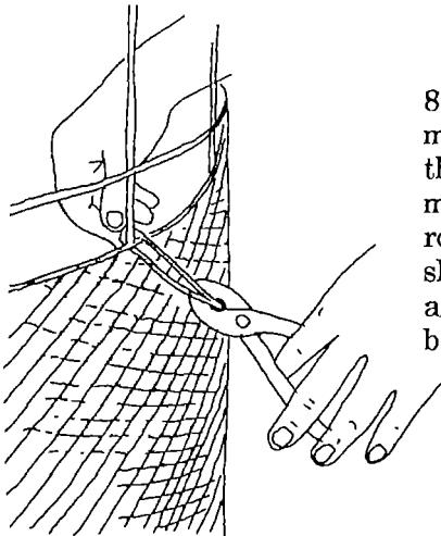
88. Wrap 2 to 3 layers of fine chicken wire mesh around the steel cage and secure it to the steel bars with soft tie wire. The wire mesh is extended up and over to cover the roof form. Carefully cut out the manhole shape and tank overflow. The manhole frame and overflow pipe are positioned and secured before plastering the tank.
