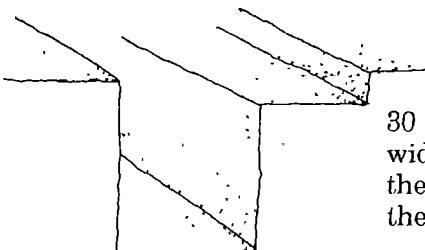
30 Excavate the foundation trench 300 mm wide and 300 mm deep. Remove any topsoil to the depth of 150 mm over the whole area of the base.
