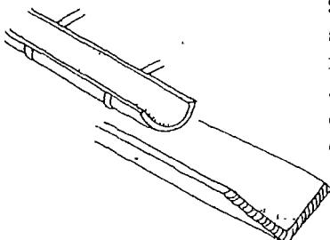
99. Gutters made from split bamboo or V shaped boards can be used to collect the rainwater from thatched roofs. The gutters are secured by straps or wires to the rafter ends, providing sufficient fall towards the outlet to drain the gutters.
