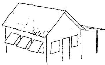
98. Rainwater collected from thatched roofs may sometimes smell of decomposed leaves and have a yellowish or tea colour. To clean the water, it can be filtered through crushed charcoal, coconut fibre or sand. For these reasons local attitudes and tradition play an important part in the use, or otherwise, of such run off.
