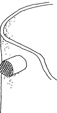
68. Cut a piece of 50 mm PVC pipe, long enough to be used as a tank overflow. Decide on the position for the overflow and cut a hole down from the top of the tank, through the tank wall. Provide the overflow level about 50 mm below the top of the wall. Carefully break out the cement and cut through the reinforcing. Fit the pipe, and cement it in place. The end of the overflow outside the tank should be screened with insect mesh.
