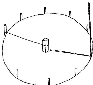
80. Around this circle, a number of 12 mm bent reinforcing *starter bars* are driven into the base. The vertical reinforcing rods are then wired onto the starter bars. This securely fixes the tank to the base.
