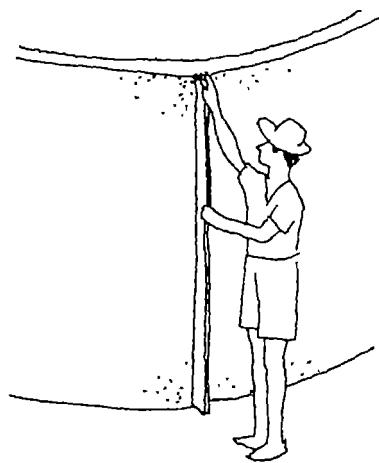
60. Using a straight edge, check the thickness of mortar between the bottom and top of the tank. Strike off any high spots. After the mortar has hardened slightly use the steel float to smooth the surface.
