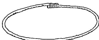
85. Circular hoops of different diameters or sizes should be formed and placed on the bottom and top of the tank. The reinforcing rods and hoops are then tied together using soft tie wire.
