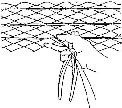
47. The hoops should be *parallel* to each other and tied to the woven mesh with tie wire at about 500 mm in the horizontal spacing. The hoops should be tight and the joins in the wire must be staggered. The hoops can be *kinked* to tighten them firmly in place.
