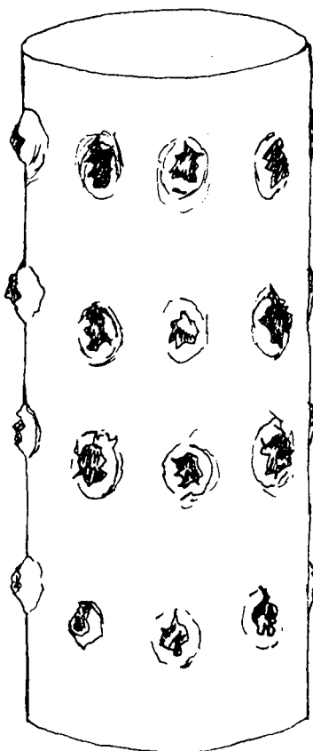
FIG. 15-5. PUNCTURED METAL CASING USED AS WELL SCREEN
