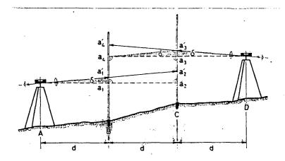
In a flat area, a stretch of about 45 to 60 m is divided into three equal lengths (d). A peg should be driven in at points B and C. Set up instrument at A. Hold staff on peg B. Take reading at a'1. Hold staff on peg C and take reading a'2. Move instrument to D. Take reading a'3 (staff on C) and a'4 (staff on B).
